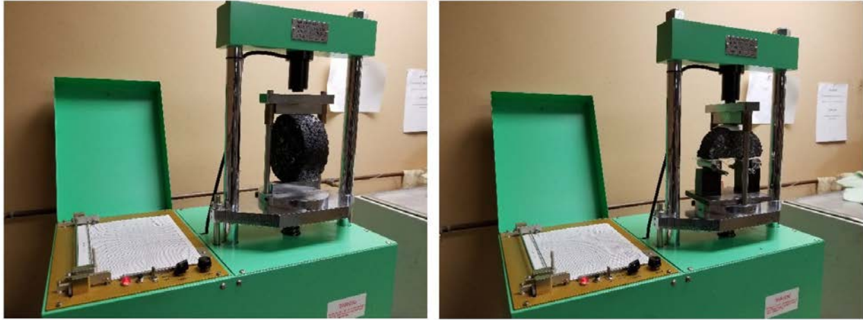
Figure 12. Marshall Compression Machine Test Set-up: IDEAL-CT Test (Left), and Semi-Circular Bend (SCB) Flexibility Index Test (Right)
